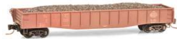
522 44 020, Reporting Marks NYC 7---05 (middle two digits of road number obscured). 50 Foot Gondola, Fishbelly Sides, Drop Ends, New York Central.
