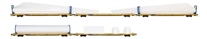
In addition to the above, the **TTX Wind Turbine Set (993 01 330, \$169.95)** has been released. UMTRR coverage was in the May 2015 issue. The individual catalog and road numbers are as follows: 071 51 810, 156656, (with blade load); 071 52 810, 156970, (no load); 071 53 810, 157213 (with blade load); 071 54 810, 157635 with load of two hubs and one engine); 071 55 810, 157697 (with tower load).
