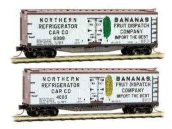
049 00 780 and 049 00 790, \$27.60 each Road Numbers: 6399 and 4000 (will be "NRC 6399" and "NRC 4000" on website listings). 40 Foot Wood Double Sheathed Refrigerator Cars, Vertical Brake Staff, Fishbelly Underframe, Northern Refrigerator Car Company / Bananas Fruit Dispatch Company.
