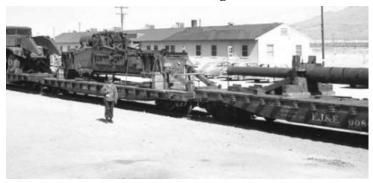
rather interesting photo on alt.binaries.pictures.rail today. Here's the description that came with it. 'January 20, 1953 - The 280-mm gun capable of firing an atomic projectile 20 miles is shown upon its arrival at Nellis Air Force Base. The weapon when assembled is 84 long, 10 feet wide. Eight flat cars were required to transport the components.'
