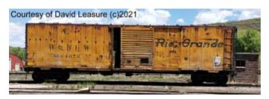
"The originally solid orange car to start was demoted to MOW and repainted into the silver MOW scheme keeping its same number. The road name and reporting marks were repainted over the silver, but not quite lining up. Over time, the silver paint faded away leaving both
